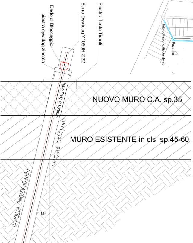
**SCHEMA ASSEMBLAGGIO TIRANTE IN BARRA DYWIDAG**
